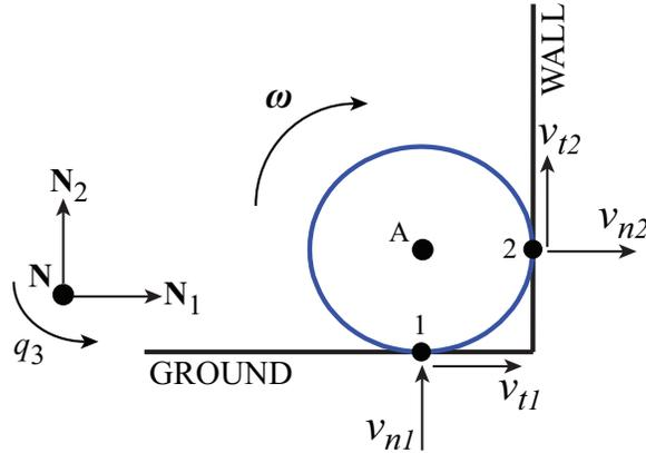
Figure 3: Velocity components at the contact points.
