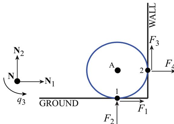
Figure 2: Contact forces at impact.
