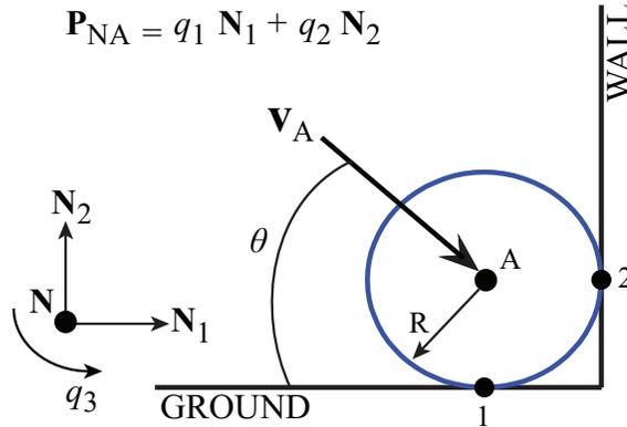
Figure 1: Planar model of a ball.
